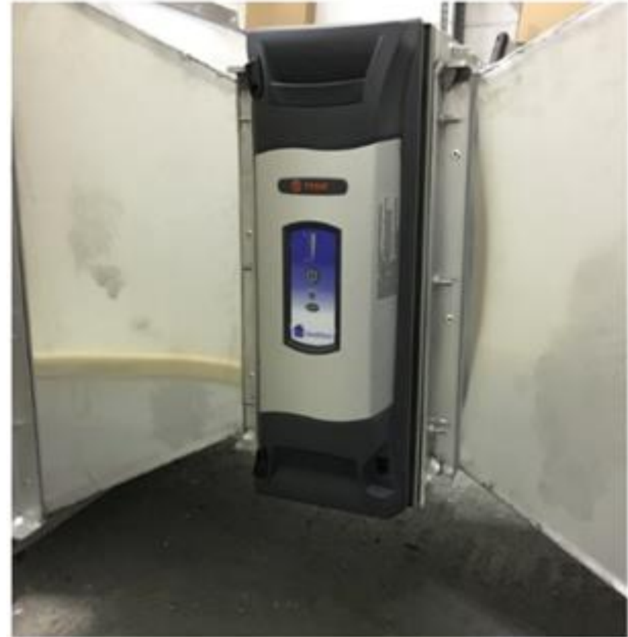
Figure 5: Electrostatic device installed in the test rig
